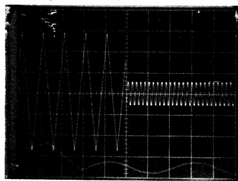
TOP TRACE: MULTIPLEXED OUTPUT 1V/DIV & 100 \mu\text{sec}/\text{DIV} BOTTOM TRACE: TIME EXPANSION OF SWITCHING BETWEEN INPUTS 2V/DIV & 5 \mu\text{sec}/\text{DIV}
